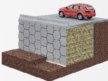
Reinforced Earth walls
